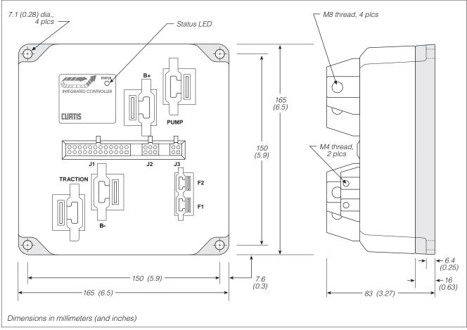
Fig. 2 Mounting dimensions, Curtis PMC 1297controller.
