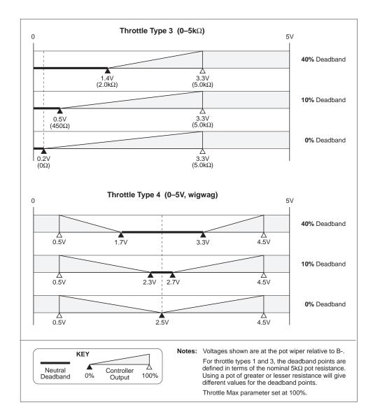
**Fig. 13, cont'd** *Effect of adjusting the throttle deadband parameter (throttle types 3 and 4).*
