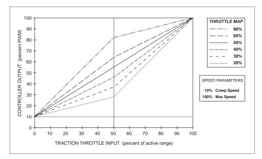
controller with maximum speed set at 100% and creep speed set at 10%.
