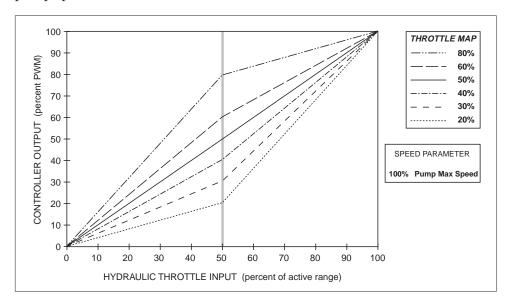
Reducing the maximum pump speed will limit the controller's output range. Throttle map profiles with the maximum pump speed reduced from 100% to 80% are shown in Figure 245. The throttle map is always a percentage of the controller's output range. So, in these examples, the throttle map is a percentage of the 0–80% output range; a 40% throttle map setting will give 32% output at half throttle (40% of 80% = 32%). Controller output will begin
