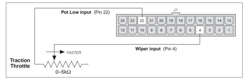
Broken wire protection is provided by the controller sensing the current flow from the wiper input (Pin 4) through the potentiometer and into the Pot Low pin (Pin 22). If the Pot Low input current falls below 0.65 mA or its voltage below 0.06 V, a throttle fault is generated and the throttle request is zeroed. NOTE: The Pot Low pin must not be tied to ground (B-).
