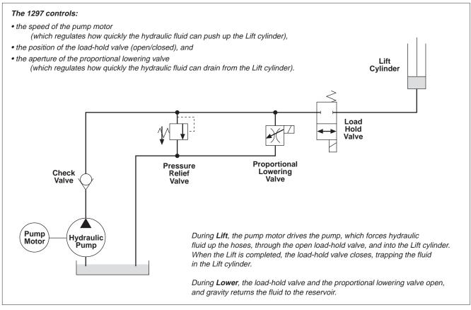
Fig. 20 Hydraulic system diagram.
