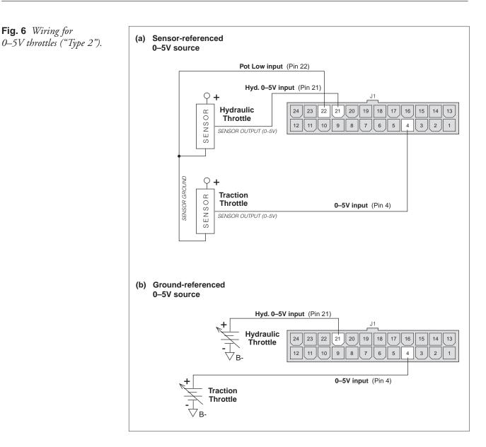
Also, the controller recognizes the voltage between the wiper input and B- as the applied throttle voltage and not the voltage from the voltage source relative to the Pot Low input.
